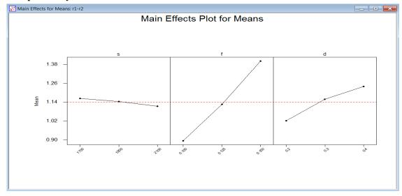
Fig: 1. Effect of turning parameters on Surface Roughness
