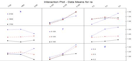
Fig: 2. Effect of turning parameters on Surface Roughness
